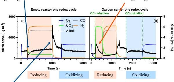
• Walls release alkali when switching to inert atmosphere
