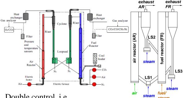
Double control, i.e. control of flows from both air and fuel reactors
