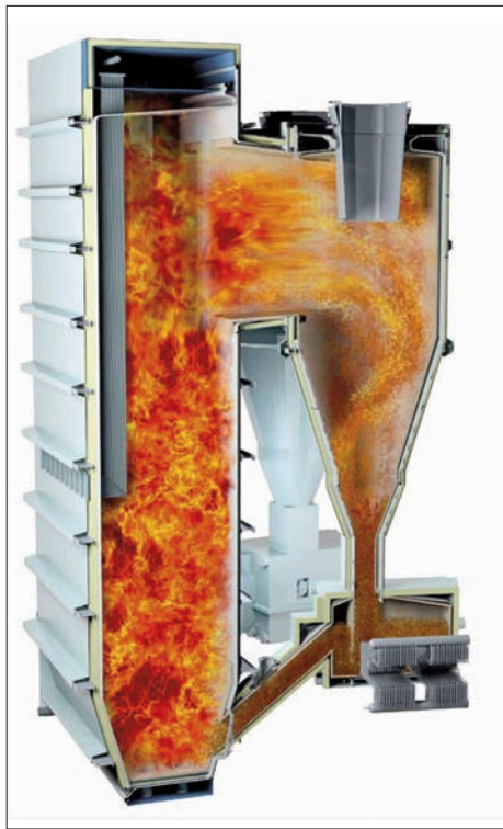
Fig. 2 - Circulating fluidized bed (CFB) boiler
