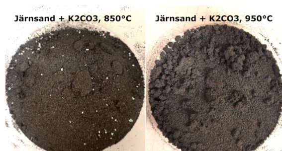
Figure 10: Photos of samples of Järnsand from fluidized bed interaction experiments with the addition of K_2CO_3 . The left photo (experiment was conducted at 850^\circ C ) shows white grains that were identified as K_2CO_3 in SEM-EDS analysis.
