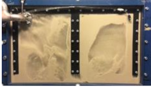
(a) 0.6 m/s, V_{sv} \sim 30\% , VD Mode 1B without Internal baffles, AD 1660
