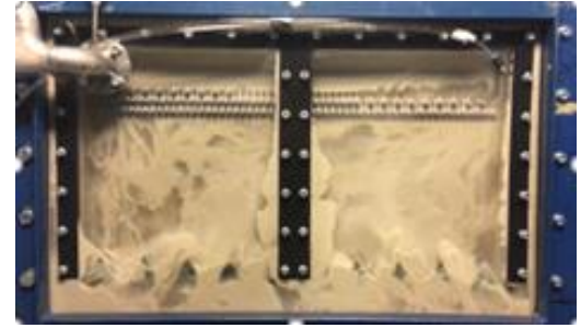
(f) 3.7 m/s, V_{sv} \sim 10\% , VD Mode 1B with Internal baffles, AD 1660
