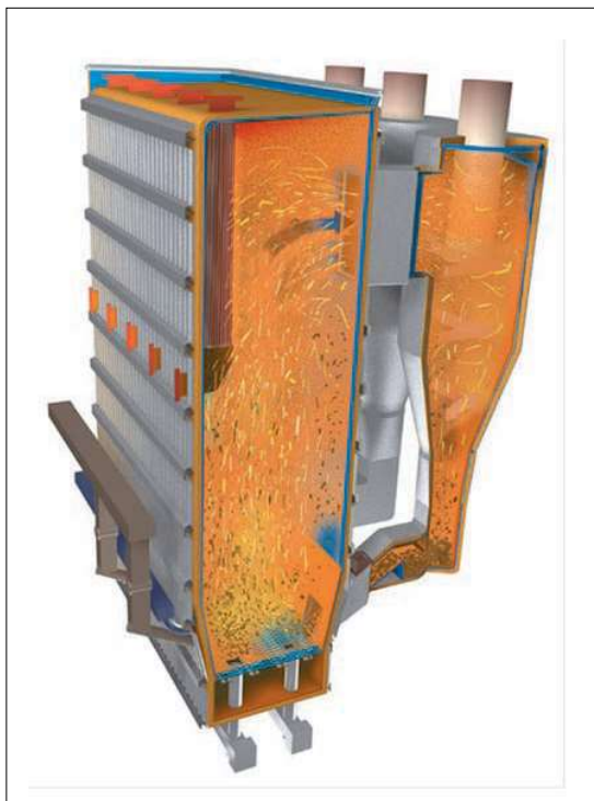
Figure 2. Circulating fluidized-bed boiler
