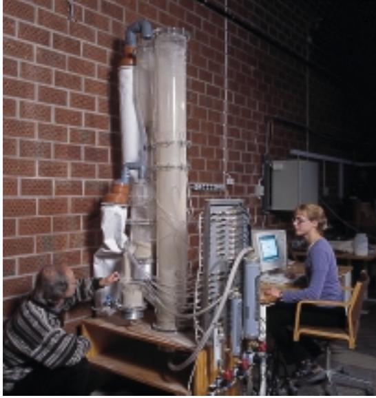
Figure 5: A perspex model of a CLC system of interconnected fluidized beds. For details see [8].
