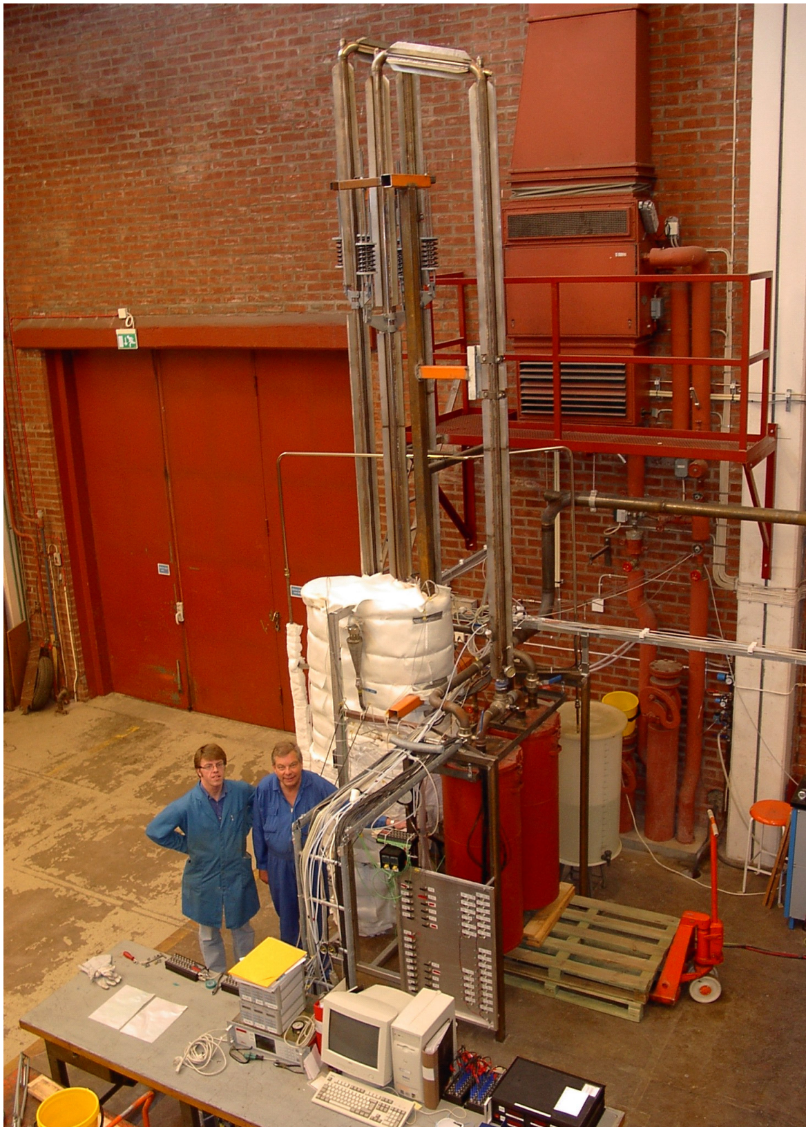
Fig. 3. Chalmers 10 kW chemical-looping combustor
