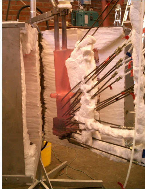
Figure 12. The hot chemical-looping combustor
