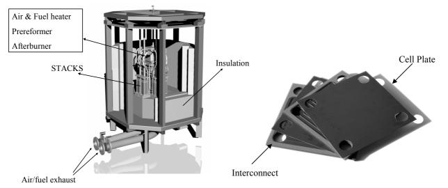
Fig.2. The Mjøllner 10 kW SOFC system. The pilot plant with STACKS and integrated balance of plant components (left). Cell plates and interconnects (right).
