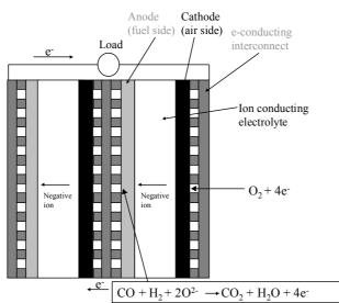
**Fig.1. Planar SOFC STACK operating principle.** Oxygen "diffuses" from the air side (cathode) and reacts with the fuel,  $H_2$  and CO, produced by reforming natural gas. The air exhaust is hot oxygen depleted-air, and the fuel exhaust consists of steam,  $CO_2$  and unburned fuel whose respective concentrations depend on the inlet fuel used and on the fuel utilization. Note, the STACK elements are not drawn to scale.
