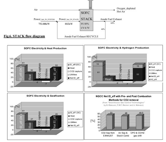
Fig.7. Energy balances for SOFC based power plants including CO2 capture
