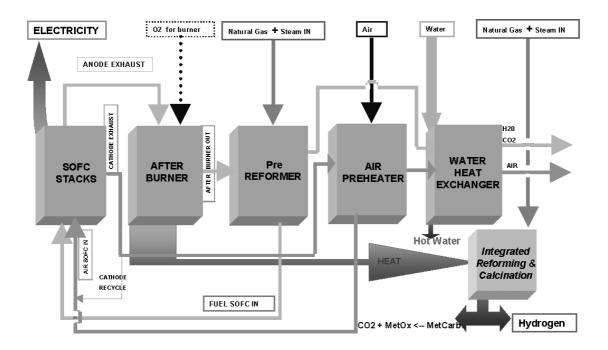
Fig.4. SOFC Power Plant - combined hydrogen & power production
