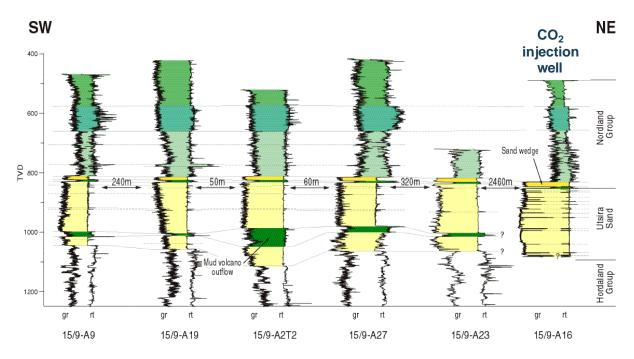
*Examples of wireline well-logs through the Utsira formation. The Utsira sand (yellow) is homogeneous, but intersected by thin discontinuous horizontal shales.*
