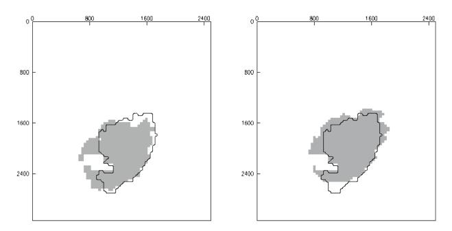
Figure 4: The CO<sub>2</sub> accumulation in the second accumulation is shown as a grey area without wind (left) and with a 3 m/year south-west aquifer wind (right). The corresponding seismic image is shown as a contour line
