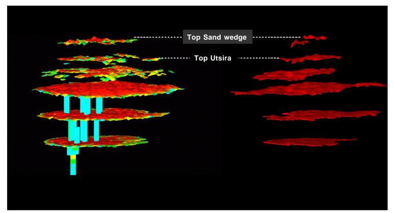
*Figure 3.* Simulated image (left) after three years of injection compared to seismic images (right). The largest bubble is approximately 1600 m long and 800 m wide. The other bubbles are approximately circular.
