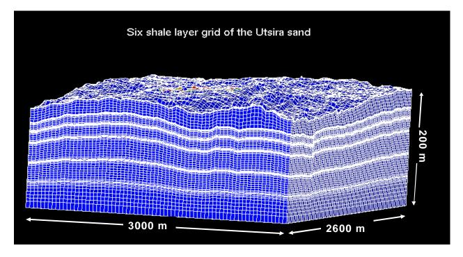
*Figure 3.* A 3D reservoir grid example used for simulation of simulations of CO<sub>2</sub> distribution. The number of grid blocks were 450 000 and 900 000 in different tests.
