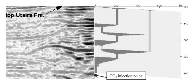
Figure 2 Left: Seismic image of a half-profile near the injection point after 3 years of  $CO_2$  injection and back-to-back (right) the corresponding simulated saturation half- profile. The diameter of the model is 1600 m.
